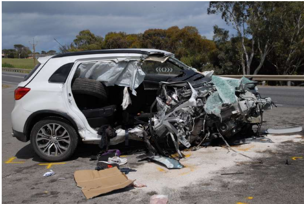
Figure 1. Damage suffered in a low overlap head-on crash on a high-speed road.
