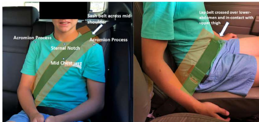
Figure 1. Good sash belt fit (sash across mid-shoulder), left, and good lap belt fit (lap belt across lower-abdomen contacting upper thigh), right. (note: Green shading indicates belt position for a good fit and red shading indicates the belt position for a poor fit)
