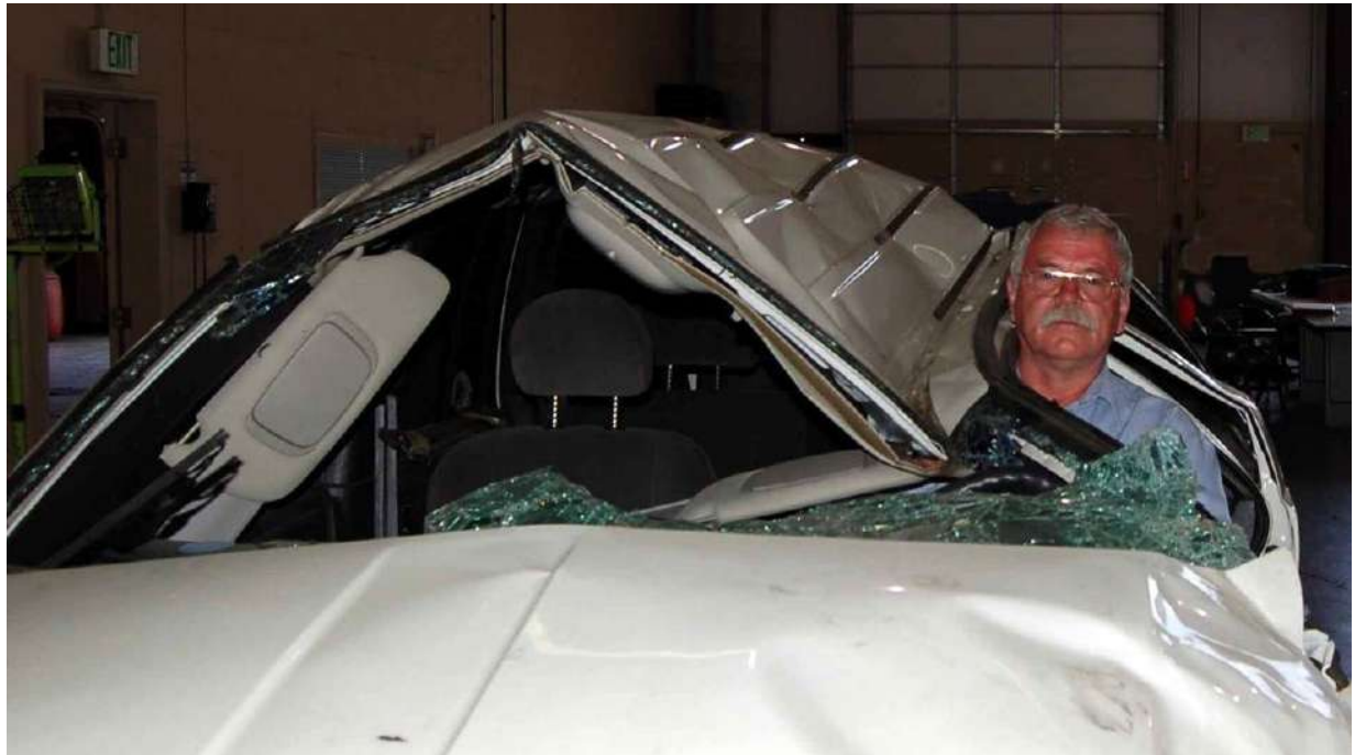
Figure 1: Poor roof strength resulting in partial ejection of occupant who was fatally injured.
