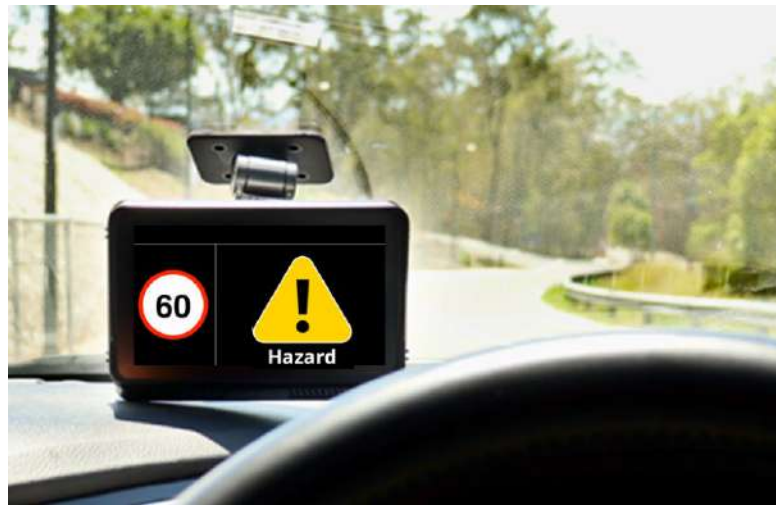
Figure 1. Dash-mounted HMI that presented alerts to participants as they drove. The example shows the display with a mockup of the in-vehicle speed and road hazard warning.
