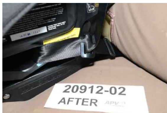
Figure 6: The gated buckle following testing, showing the partially unthreaded belt.
