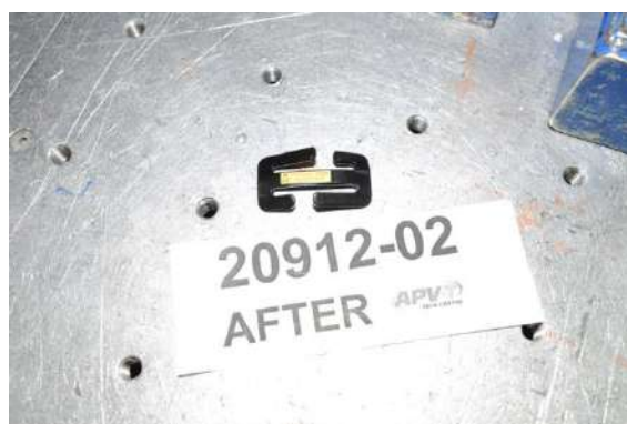
Figure 7. The bent gated buckle following testing.
