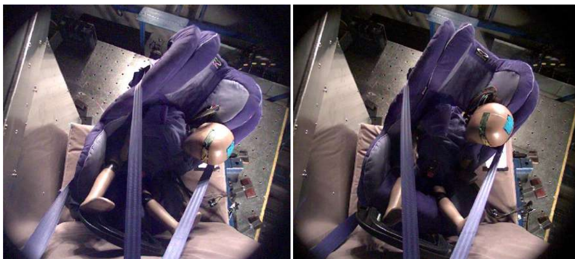
Figure 5. Dummy position during testing without the gated buckle (left) & dummy position during testing with the gated buckle (right)
