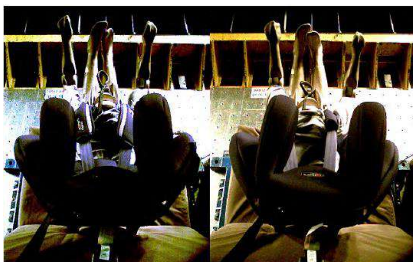
Figure 3. The backrest twisted more during the gated buckle test (right) when compared to the baseline test (left), at 96ms after impact.
