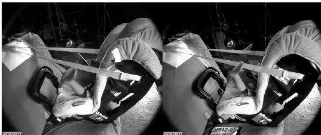
Figure 4. The restraint twisted less during the gated buckle test (right) when compared to the baseline test (left), at 96ms after impact.
