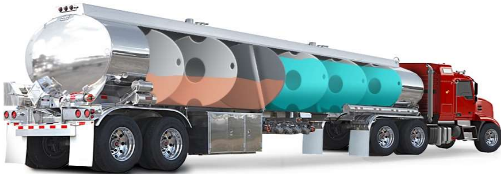
Figure 1. Baffle plates inside a road tanker
