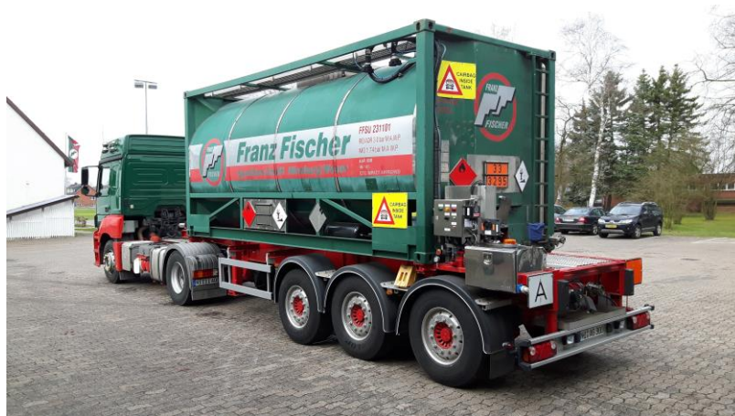
Figure 1. First “ADR” (see Reference ) tank-truck with liquid load securing “Cairbag ® ” system in Germany
