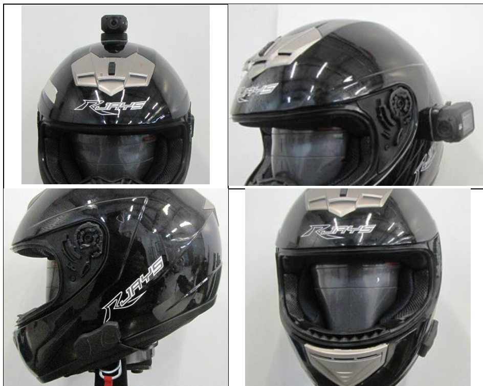
Figure 1. Examples of mounting camera and communication device onto the helmet
