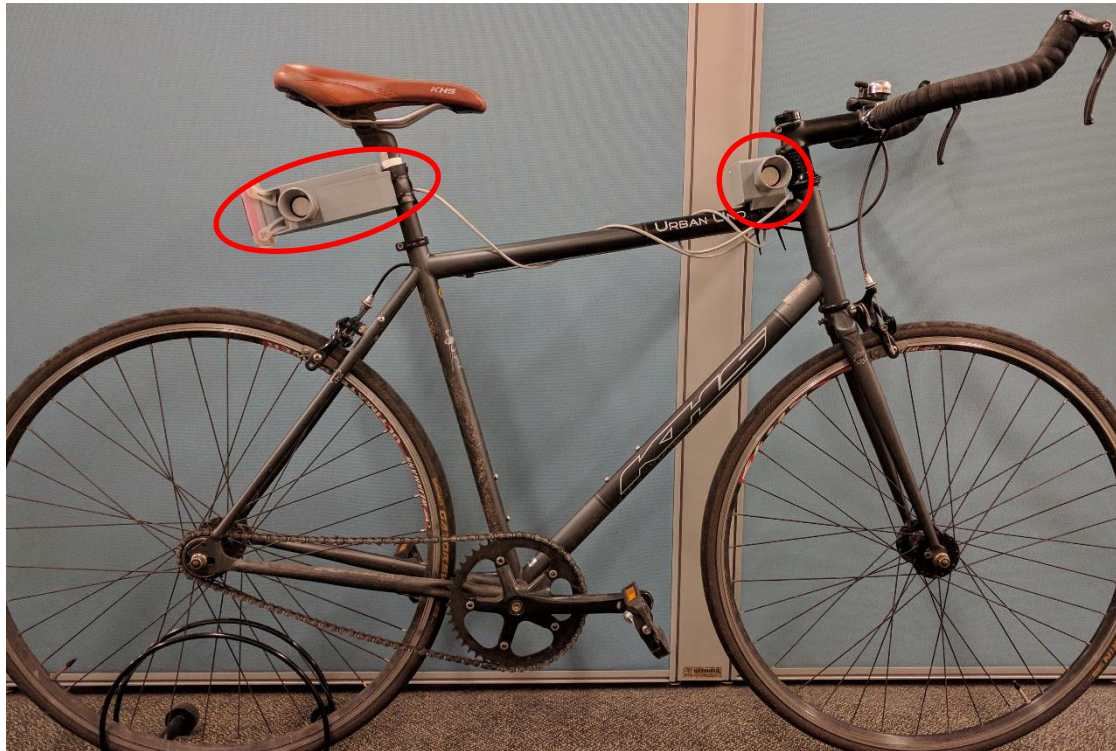
Figure 1. Passing device (circled in red) attached to a bicycle
