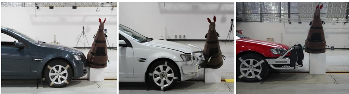
Figure 1.1 Sedan with (L-R): no bull bar, low dummy; urban bull bar, low dummy; rural bull bar, high dummy
