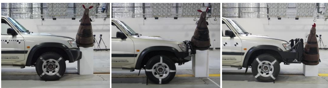
Figure 1.2 4WD with (L-R): no bull bar, high dummy; urban bull bar, high dummy; rural bull bar, low dummy
