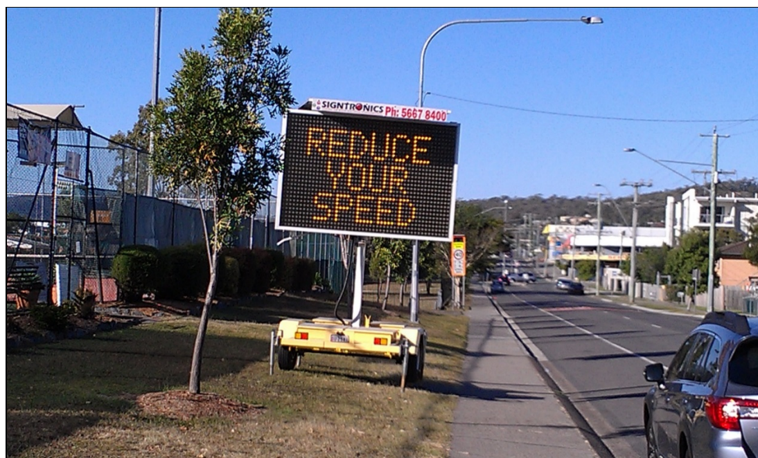
Figure 1. VMS prior to school zone showing one of the messages
