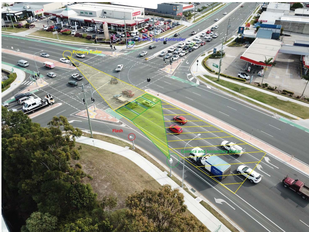
Figure 2. Labelled diagram of Hold the Red system in Ashmore, Queensland
