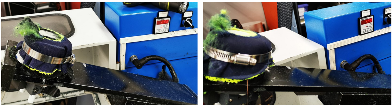
Figure 1. Abrasion testing shown here on the summer jacket provided 2.52 seconds of resistance (left). Experiments that added an additional layer of fabric almost doubled that time to 4.49 seconds (right). This information was conveyed to the manufacturer.
