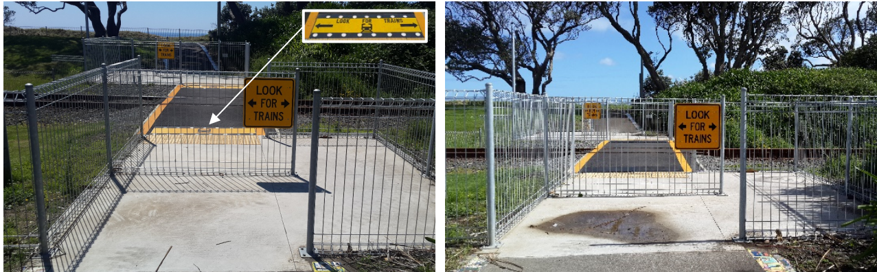
Figure 1. View of the level crossing (Left: Trial configuration (with in-ground lights); Right: Standard (control) configuration)
