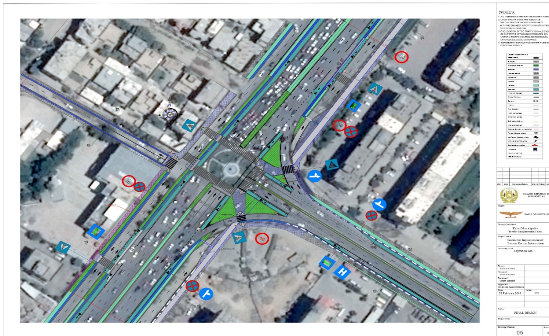
Figure 2. Example of Redesigning a circulatory intersection to a Signalized Intersection in Kabul city, Airport Road, Layout on GIS map, Saleem Karwan Intersection
