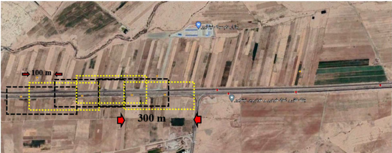
Figure 1. Identifying high-crash sections using sliding window method
