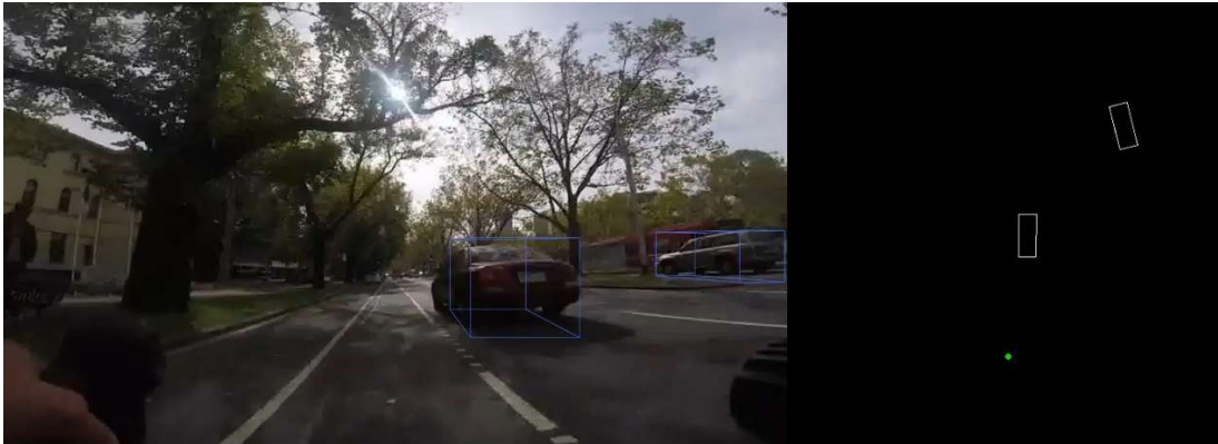
Figure 1: Example of the detection of passing vehicles using on-bike video data
