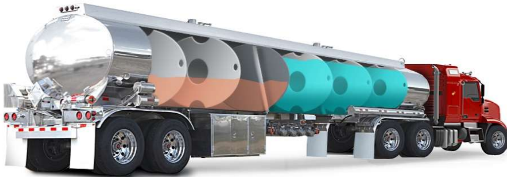
Figure 1. Baffle plates inside a road tanker
