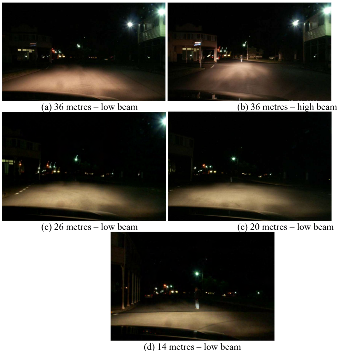
Figure 2: Visibility of pedestrian at various distances from the vehicle, standing in the middle of the road, at the intersection close to where the pedestrian was struck.
