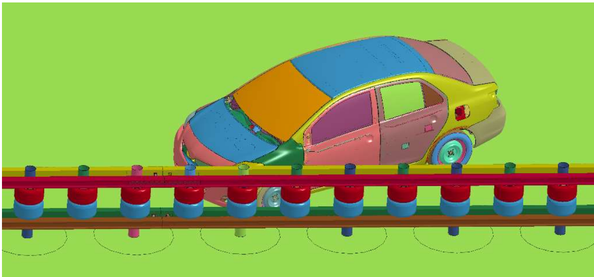
Figure 1. Finite element model of Toyota Yaris crashing into a segment of safety roller barrier
